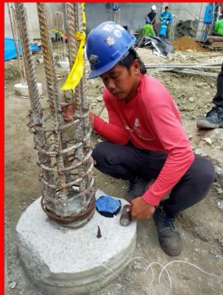
Testing: Pile Integrity Test and High Strain Dynamic Load Tests, (PDA Test) c/o C.G. Integra at Brgy. Banga 1st Ground Reservoir Project
