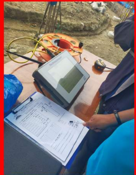
Testing: Pile Integrity Test and High Strain Dynamic Load Tests, (PDA Test) c/o C.G. Integra at Brgy. Banga 1st Ground Reservoir Project
